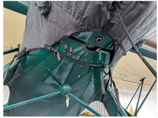
Wacon Cabin Biplane ZQC-6 Insulated Engine Cover
