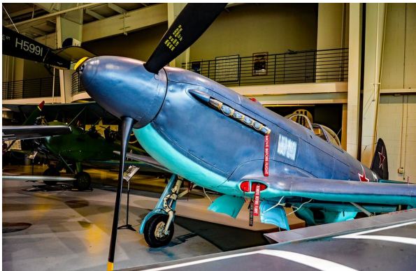
Yakovlev Yak 3 Oil Cooler Inlet Plugs
