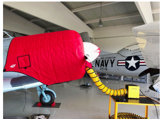
Yak 11 Insulated Engine Cover
