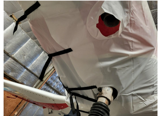
Zlin 142C Engine Cover, test fit cover
