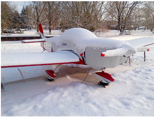
Zenith 601XL Canopy, Prop/Spinner and Insulated Engine Cover
