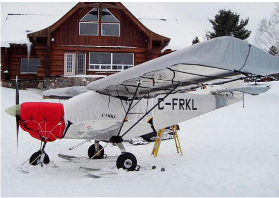
Zenith 801 Insulated Engine, Canopy, Wing & Tail Covers
